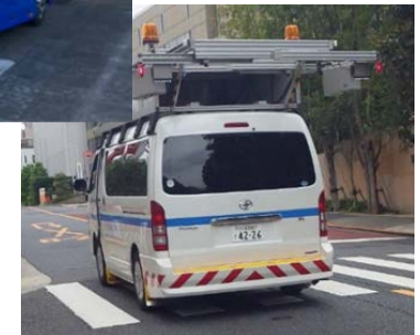
A vehicle that measures pavement surface profiles
