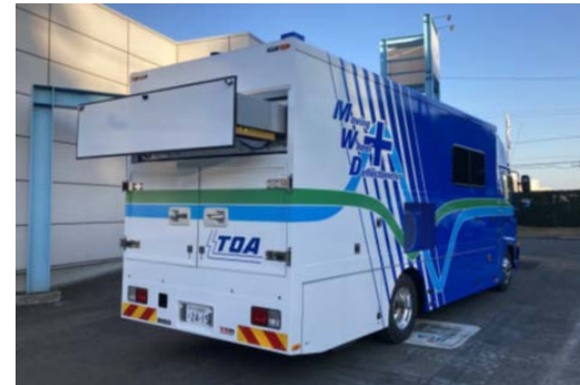
Mobile deflection measurement equipment MWD plus
