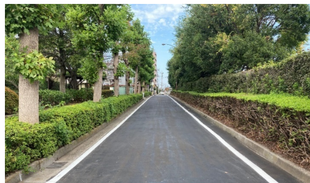
Road paved with cold-mix asphalt (Nerima City, Tokyo)
